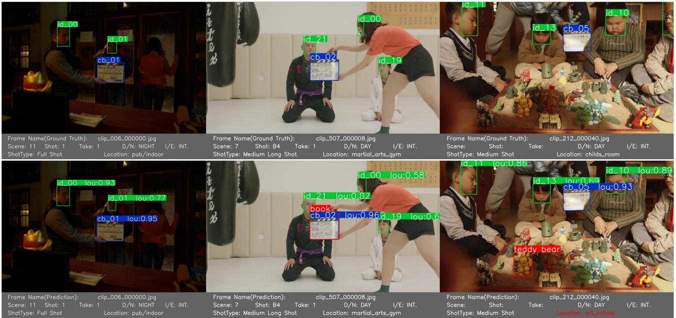
Figure 5: Region predictions and semantic annotations on Film-RVSAD. We use our method to generate metadata for video search and retrieval. Examples in the upper line are ground-truth in Film-RVSAD, and examples in the bottom line are results from our proposed system.
